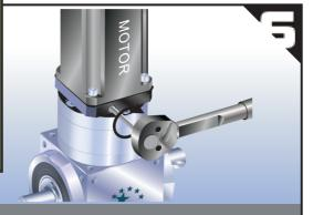
Tighten the set collar bolt with torque wrench to specified torque. (See Table 2)
