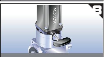
Tighten back the screw plug.
