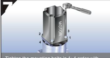
Tighten the mounting bolts in 1~4 order with torque wrench to specified torque. (See Table 1)
